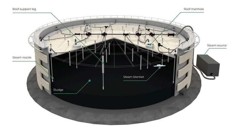
Steam is supplied into the oil sludge through specially designed steam nozzles
