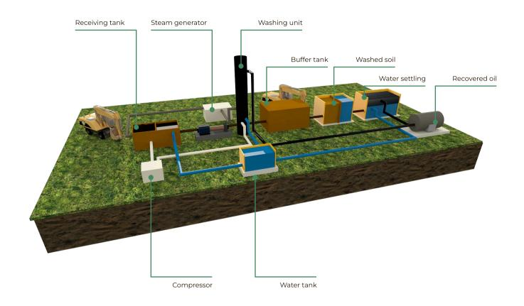
This technology is used to treat oil-containing soils, sandy soils and loam soils. Oil-contaminated soils are washed by the special unit designed and developed by Arkoil. Oil-contaminated soils are homogenized. After being treated by compressed air, water and steam, homogenized material is separated into three fractions.
