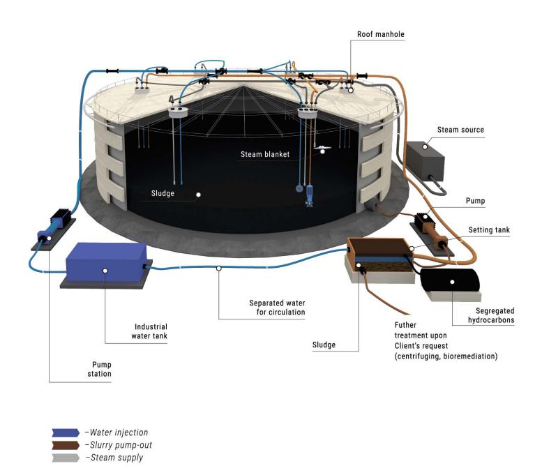
The system is applicable for tanks containing sludge with high content of asphaltens, sulphur or low content of hydrocarbons, and also for heavy oil tanks.
