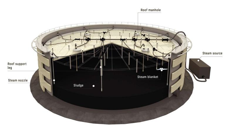
Steam is supplied into the oil sludge through specially designed steam nozzles
