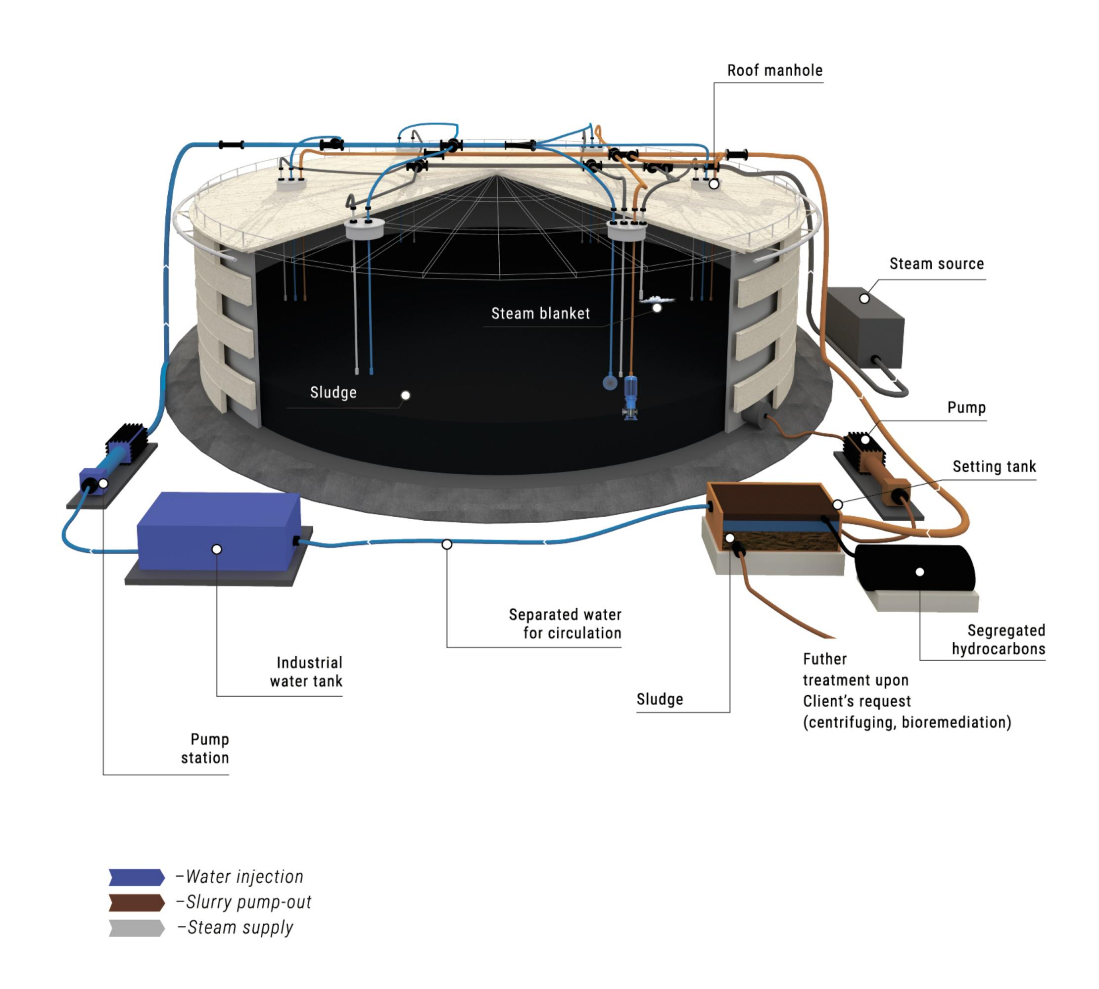
The system is applicable for tanks containing sludge with high content of asphaltens, sulphur or low content of hydrocarbons, and also for heavy oil tanks.
